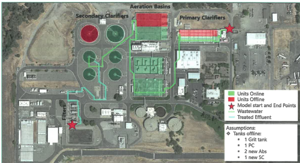
FIGURE 3-6: DCWWTP AERIAL WITH HYDRAULIC MODEL FLOW PATH
